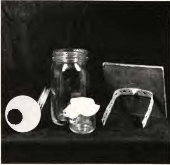
Fig. 2. NIT trap made of a 1-quart wide mouth canning jar with a funnel, an isolated bait container, and a rain cover. The cover is held in place with duct tape.
